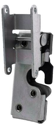
This single rotor latch is a sub-platform to the TriMark proven 050-0400 series latch and is designed for medium to heavy-duty applications for on or off highway compartments and access panels. It features a coaxial trip mechanism for applications where it is desirable to provide additional support to the trip lever and is FMVSS 206 (ECE R11) compliant.
